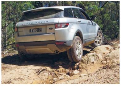
Top: The front left wheel is spinning, but neither rear wheel is rotating, hence we're going nowhere. This shouldn't be possible, and is akin to driving a Discovery 2 or Defender with the centre diff unlocked. The 4x4 system should send more torque to the rear wheels, and the vehicle should only fail to proceed when one front and one rear (usually diagonal) wheels have lost traction. The rear wheels have weight on them, so should have more torque to make use of the traction
