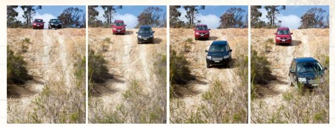
Same race, but HDC not engaged on the Freelander. This shows how much braking HDC has to do in order to compensate for the lack of low range. The more braking, whether by computer or human, the greater the chance of a skid.
