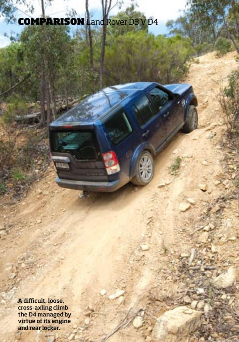
A difficult, loose, cross-axling climb the D4 managed by virtue of its engine and rear locker.
