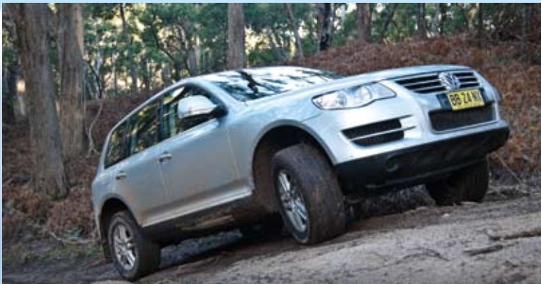
On this slope the Touareg's stiff suspension could not apply sufficient weight to the wheels to permit progress without the traction control needing to assist.
