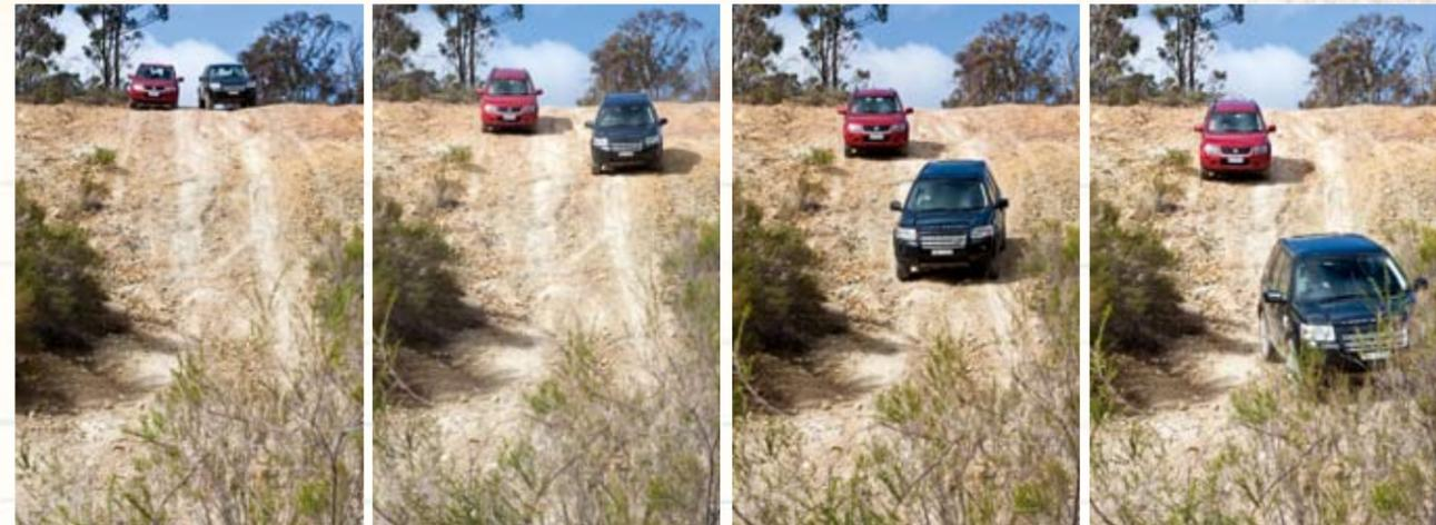
Same race, but HDC not engaged on the Freelander. This shows how much braking HDC has to do in order to compensate for the lack of low range. The more braking, whether by computer or human, the greater the chance of a skid.
