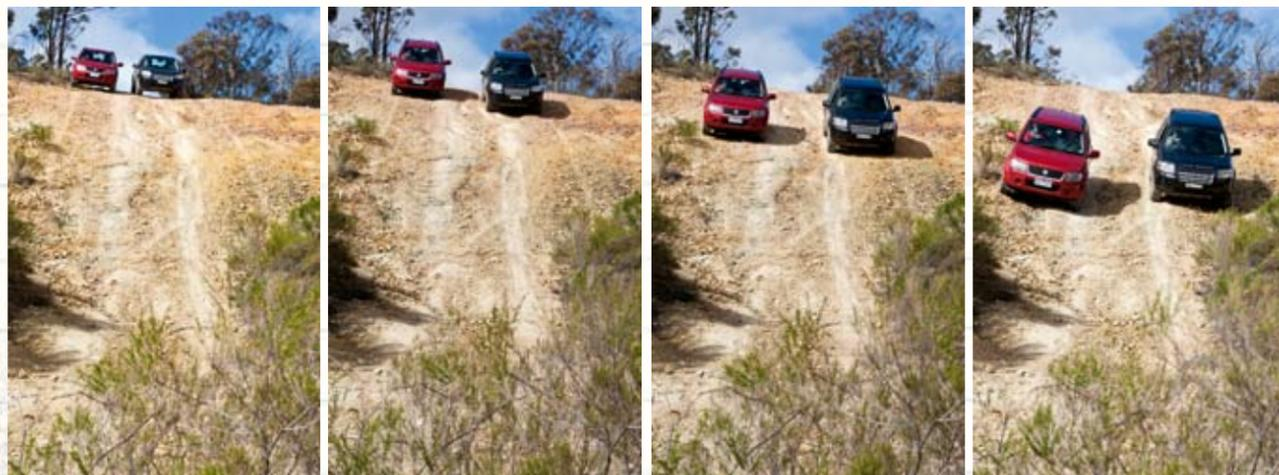
Starting at the top; Freelander has HDC engaged, Suzuki first low, feet off the pedals. See main body for commentary.
