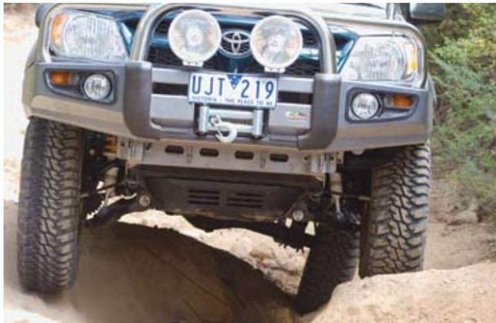
**Leaf springs rear and independent-front are never going to provide the ultimate in flex, so it's important to maximise what travel there is through low-friction leaves and careful choice of springs and shocks.**
